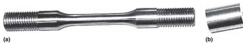
Fig. 1 Specimen configurations: (a) smooth tensile specimen and (b) electrochemical polarization specimen
